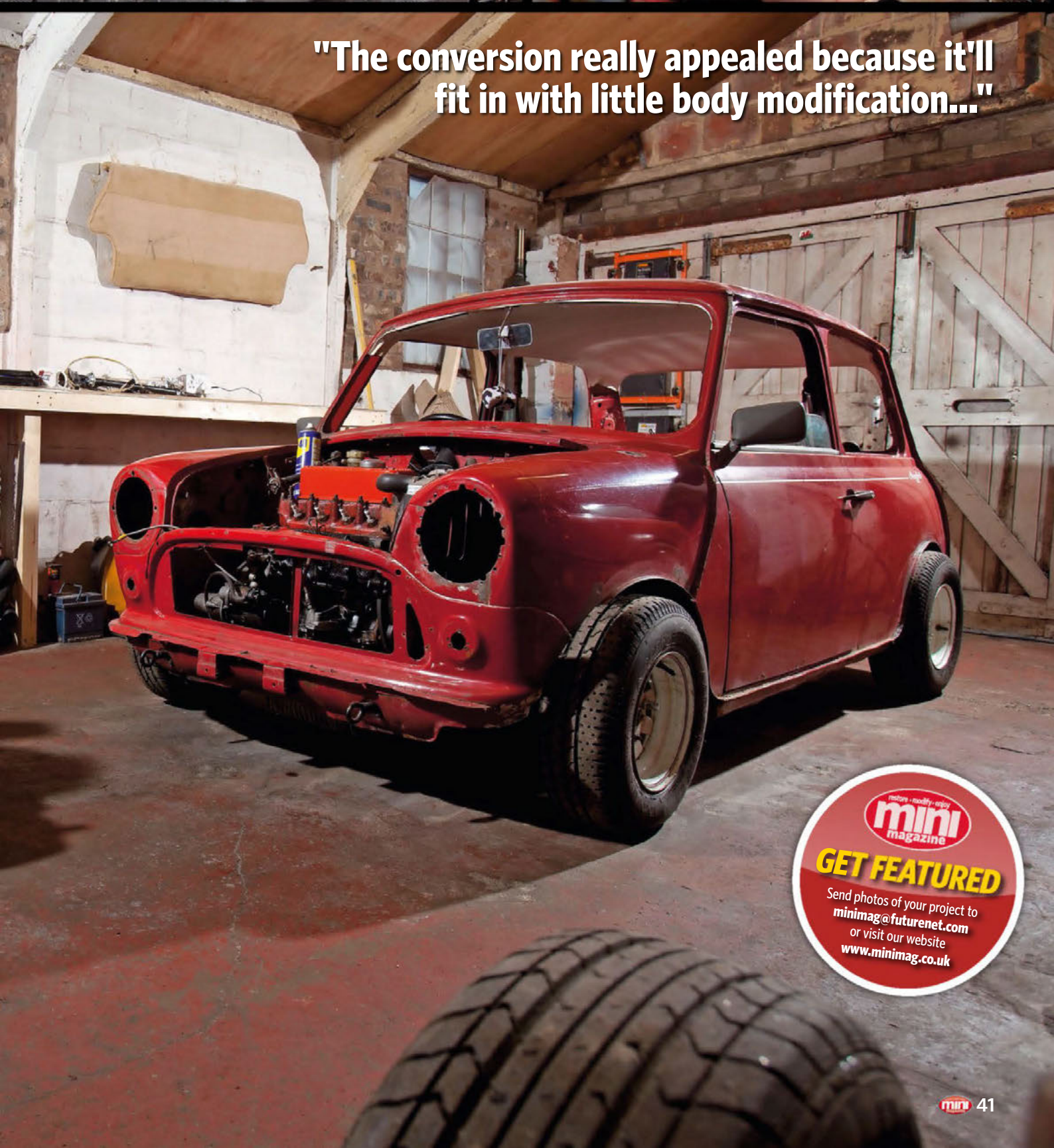
The head came from a 130bhp BMW K1200RS motorbike, made from '97-'05.
