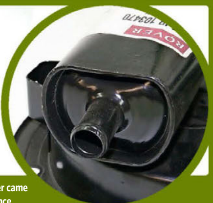
Large-bore solid-wall blocks (no tappet chest cover plates) have a breather fitted to the timing cover. The Cooper S never had one, only the 1275 GT in a Mini where space between the cannister and fan blade wasn't an issue, allowing a wide spacer to be fitted to move the fan blade well away from it.
