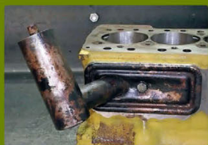
OE breathers are well designed and usefully positioned. Small-bore and 'real' Cooper S blocks have tappet chest cover plates on the back, perfect for the factory made component.
