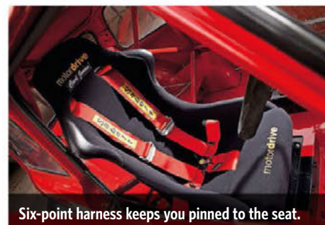
Nothing but the bare essentials here - seat, harness, switch panel and the incredibly intricate weld-in 'cage'.
