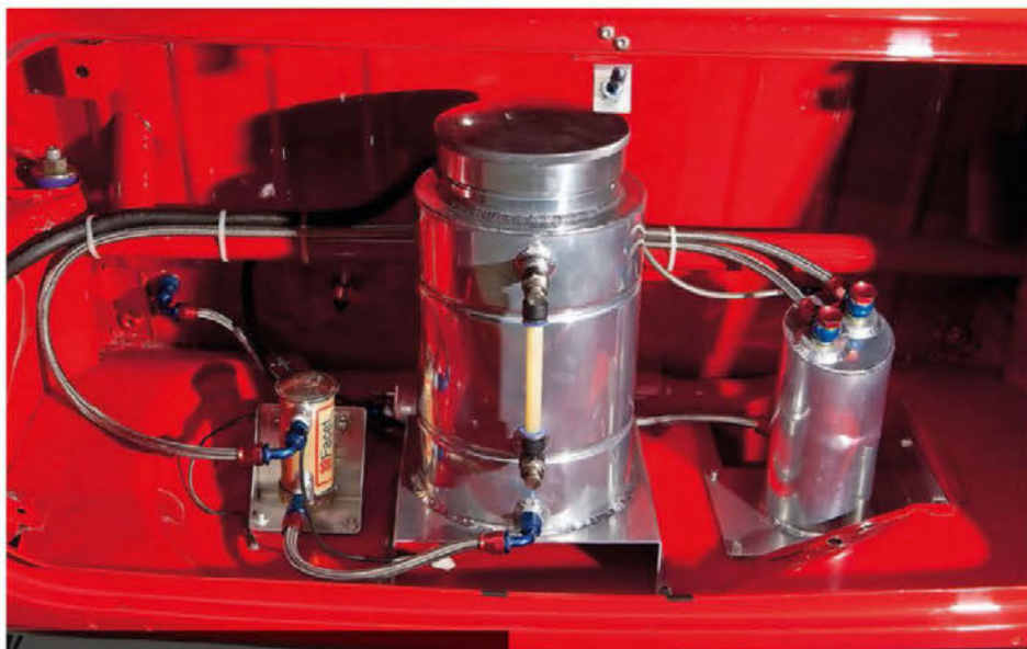
Two-gallon fuel cell is all that's required for short runs. Swirl pot is essential for the injection set-up.
