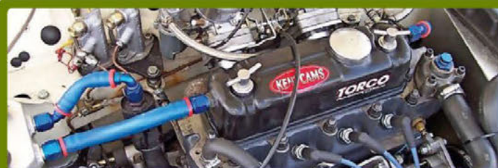
The catch tank needs to be on right hand side, preferably as high as possible. This will prevent as much oil being pushed in to the catch tank as possible. Fitting it low down will allow oil to fall out to the air, stick to the pipe walls and run down into the tank. And if there is a lot of oil being forced in to the pipe, syphoning may occur. That's not at all good. This is my Clubby racer's set-up. Note the connection on the rad end of the rocker cover. This comes up from the timing chain cover. It's a neat and tidy set-up that works perfectly well.
