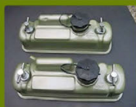
Some say just one breather is sufficient. Piston ring seal must be perfect to get away with this though. The Aussie Minis were equipped with a very neat solution on the rocker cover.
