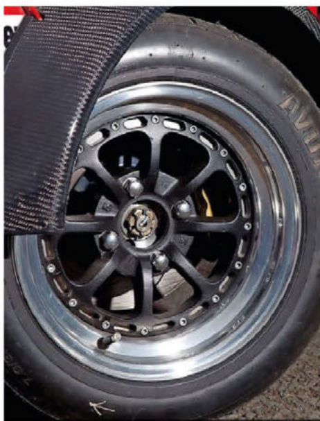
MB 13-inch magnesium split rims with Avon tyres.
