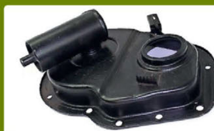
Large-bore solid-wall blocks (no tappet chest cover plates) have a breather fitted to the timing cover. The Cooper S never had one, only the 1275 GT in a Mini where space between the cannister and fan blade wasn't an issue, allowing a wide spacer to be fitted to move the fan blade well away from it.
