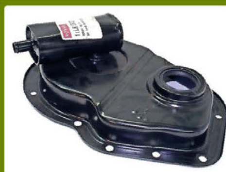
When 1275 units were fitted to round-fronted Minis, Rover came up with a flattened cannister to give the necessary clearance.
