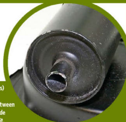
1275 units also had a breather cannister fitted to the top of the transfer gear casing. Several versions became available as room was needed to clear the servo-mounted master cylinder assembly.
